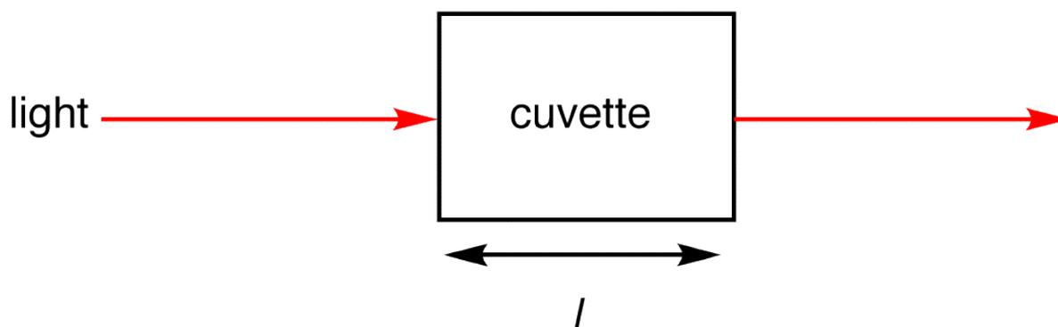
Figure 1: Light absorbed by sample in a cuvette
